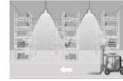
With insufficient ambient light, the sensor switches on the lamp when motion is detected.
